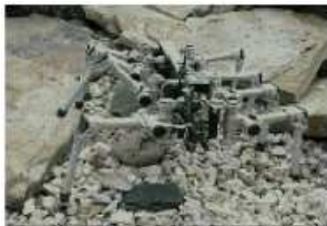
(e) Eight-legged robot Skorpion (9,5 kg). Inst. for Autonomous Intelligent Systems (AiS), Sankt Augustin.
