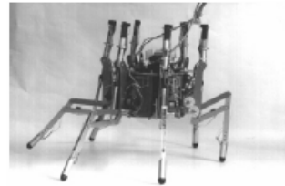
(f) Six-legged robot Silex (15 kg). Free University, Brussels.
