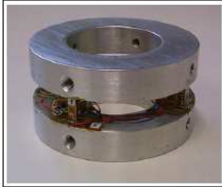
Fig. 3.6. Three-component force sensor for high loading.
