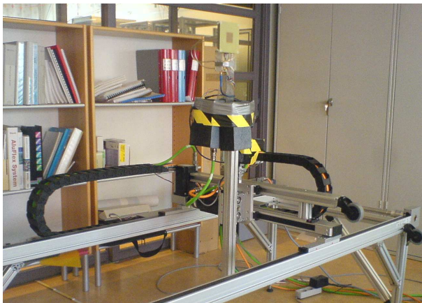
Figure 3.4: 3-D positioning robot with rotational RX probe antenna.
