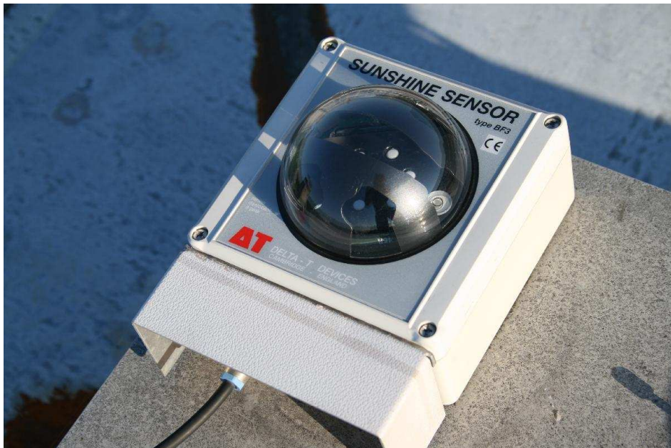
Figure 3.10: Delta-T BF3 sunshine sensor. A shading mask ensures that at least one of seven photosensitive diodes is always lit by direct sunlight, and at least one is shaded from it. The sensor can thus determine the diffuse and global components of daylight, and does not require any polar alignment (Delta-T Devices Ltd, 2006).
