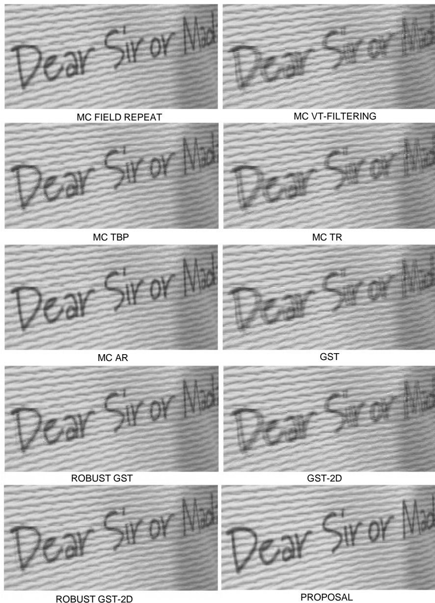
Fig. 13. Deinterlaced images obtained with MC de-interlacing algorithms and our proposal in the Paper 3D hybrid sequence.
