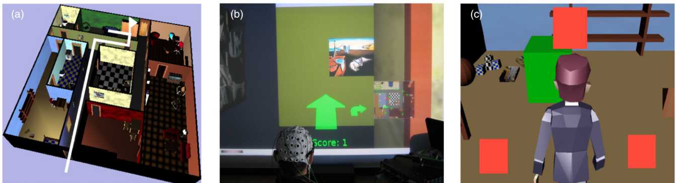
Figure 1. Two different ways to use a BCI to navigate through a virtual apartment in VR. Panel (a) presents an overview of a virtual apartment and (b) shows an image of a subject navigating through that virtual apartment with motor imagery [46]. Panel (c) shows an SSVEP BCI that can allow an avatar to move through an apartment or other environment [53].
