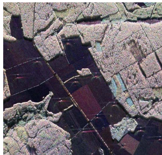
Fig. 15. Rotating windmills close to some forested areas. Image acquired by F-SAR in L-band with 1.5 \times 0.5\text{-m}^2 resolution (blue: VV polarization, red: HH polarization, green: HV polarization).
