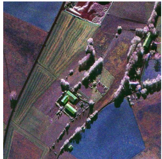
Fig. 12. Fully polarimetric F-SAR X-band image with 25-cm spatial resolution (blue: VV polarization, red: HH polarization, green: HV polarization). Building shapes and surface textures are clearly visible.
