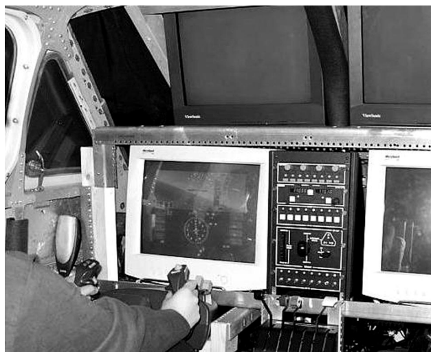
Figure 1. The flight simulator consisted of four display screens, controlled by two computers. Two screens were located on the upper row and the other two on the lower row. The left screen on the lower row was used, and the remaining screens were turned off. A pilot seat was located in front of the screen, and the yoke was placed between the screen and the seat.
