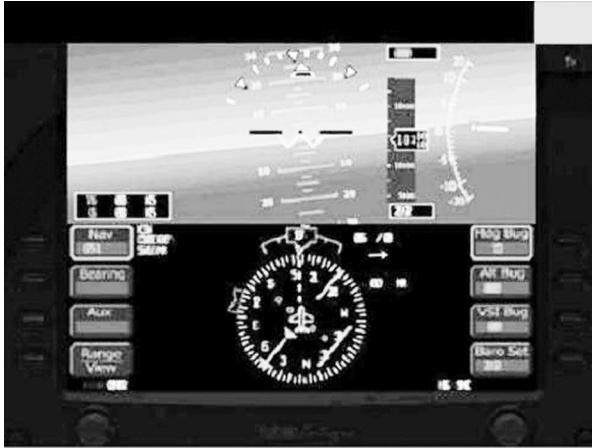
Figure 2. The inside-out format of the glass cockpit frame used in Experiment 1. The artificial horizon and the bank angle markings rotated to the left or to the right in the direction opposite to the yoke turn, whereas the aircraft symbol and the roll pointer were stable. The imperative stimulus appeared at the left or the right upper corner (a right stimulus is shown in the current figure).
