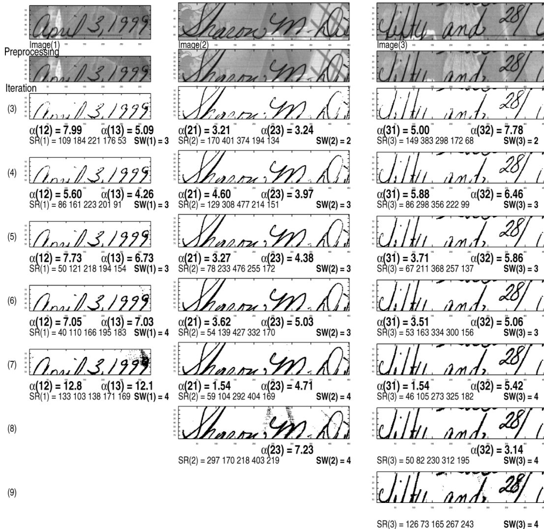
Fig. 2. Three subimages and their binarization at a sequence of candidate thresholds.
