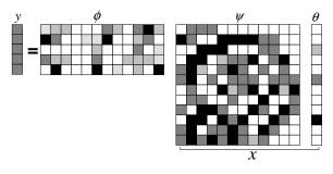
Fig. 2. Compressed sensing linear measurement process.
