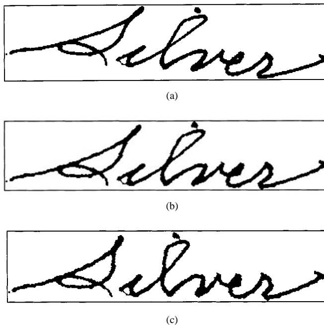
Fig. 11. Tilt and slant correction. (a) Before tilt correction. (b) After tilt correction. (c) After slant correction.
