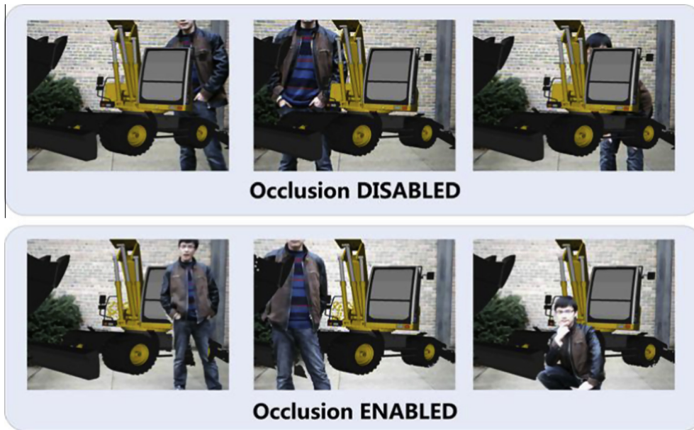
Fig. 7. Occlusion effect comparison using homography mapping between the TOF camera and the RGB camera.
