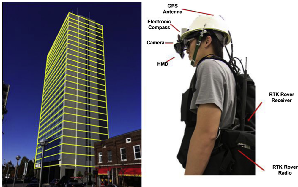
Fig. 10. Schematic overview of the designed AR-assisted assessment methodology.
