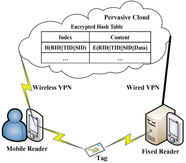
Fig. 4. The proposed cloud-based RFID authentication scheme
