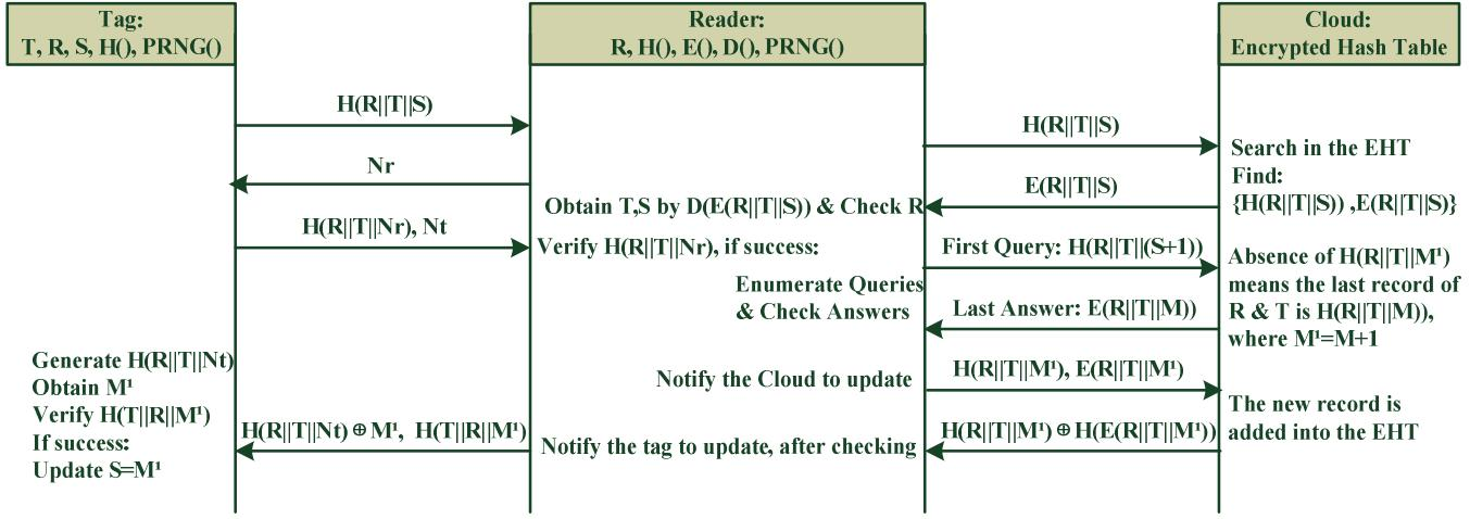
Fig. 6. The proposed cloud-based RFID authentication protocol
