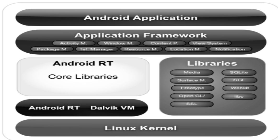
Fig. 7. Adaption of Linux kernel by Android with added additional features
