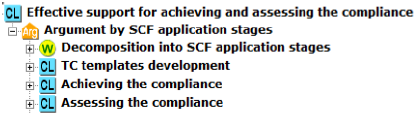
Fig. 6. First level of decomposition. Arguing SCF effectiveness by demonstrating possibility of developing sound TC templates which positively influence the process of achieving the compliance and increase efficiency of the assessment.
