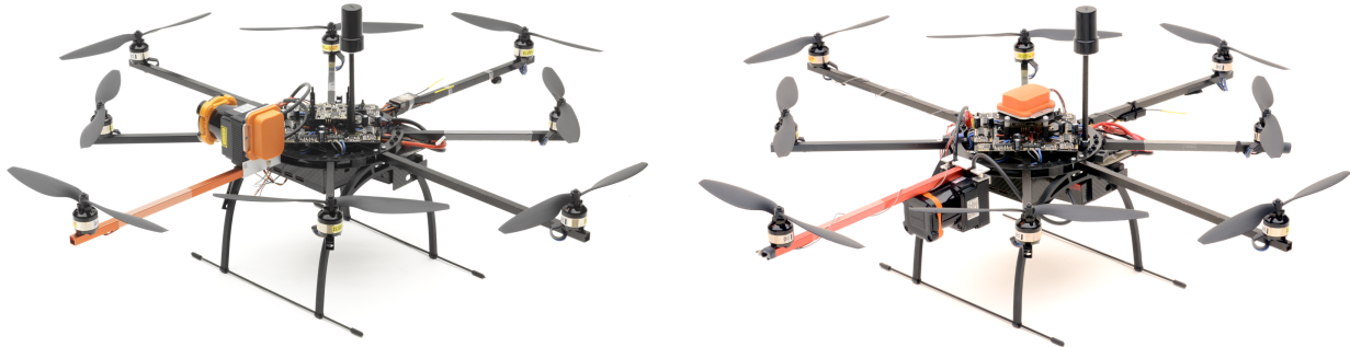
(a) First configuration, in which laser scanner’s FOV is oriented vertically and the inertial measurement unit is fixed to the scanner for precise alignment.
