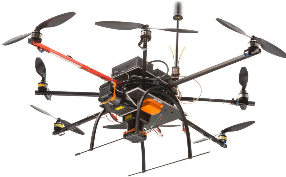
Figure 3: The current setup includes a second laser scanner for obstacle avoidance and mapping. Both laserscanners and the IMU are mounted together with the battery on a stiff and lightweight carbon-fiber sandwich-board. The resulting module makes up 40% of the UAV's weight and is fixed to the vehicle's frame using vibration dampeners. This yields less drift in the INS solution, more precise sensor alignment and better crash survivability.
