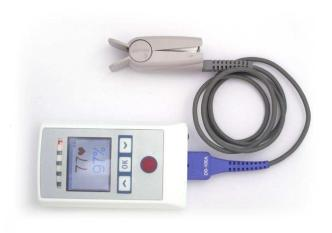
Fig. 2. Medical information tag, or miTag for short, used in MEDiSN [43]. The miTag is a Tmote mini [53] based patient monitor that includes a pulse oximetry sensor with LEDs, buttons and a LCD screen. The miTag is powered using a re-chargeable 1,200 mAh 3.7 V Li-Ion battery and external finger tip sensors are used to make the pulse oximetry measurements.
