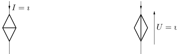
Figure 4: Controlled sources: Voltage/current controlled current source ( I = i(U_{control}, I_{control}) ), voltage/current controlled voltage source ( U = v(U_{control}, I_{control}) ).
