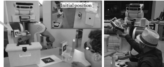
Fig. 4 (a) PR2 robot shows an object to the human, while ensuring that the object is maximally visible to him. Note that it also maintains the symbolic front and top of the object from the human's perspective. (b) PR2 robot gives an object to the human, at a place easily reachable to him, also ensuring the grasp feasibility of the object by him
