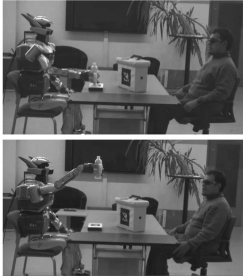
Fig. 5 HRP2 robot shows a hidden object to the human, by holding it at a place that requires the human to put least effort to see it
