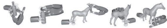
Fig. 3 Reasoning on the possibilities of the simultaneous grasps of different objects by two agents (by the robot's gripper and anthropomorphic hands) for the tasks requiring object hand-over
