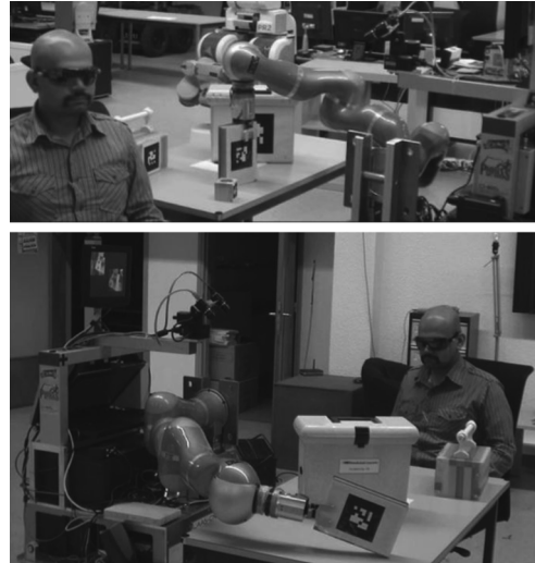
Fig. 7 Jido robot hides an object. It also shows the interesting aspect of grasp-placement interdependency. The selected grasp in initial scenario (top), facilitates the final computed placement, to place the object by a different contact facet to make it completely hidden from the human's perspective (bottom)
