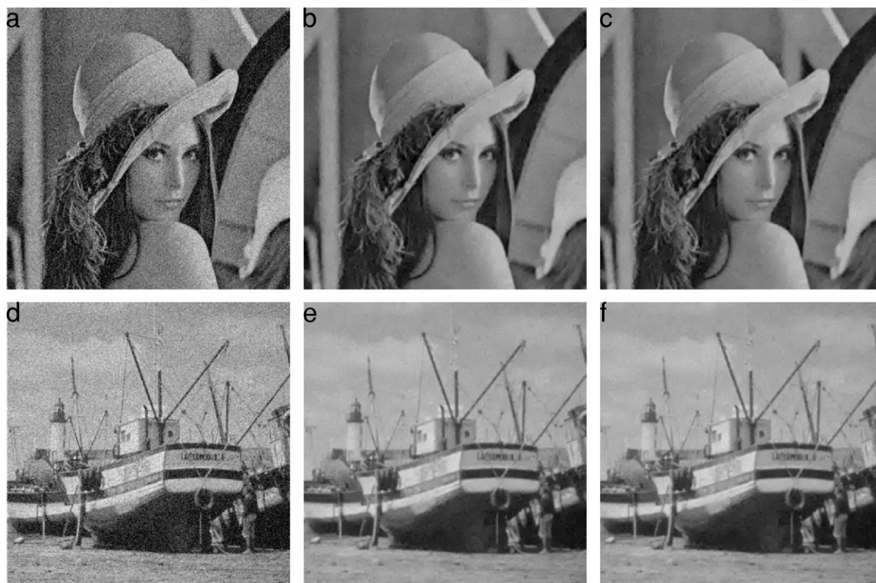
Fig. 5. Denoising results obtained with: (b), (e) the non-convex potential function PM 2 ; (c), (f) the convex potential function Ch: (a) Noisy image \sigma = 30 ; (b) PSNR = 29.51; (c) PSNR = 29.44; (d) Noisy image \sigma = 30 ; (e) PSNR = 27.55; (f) PSNR = 27.40.
