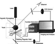
linked to a streptavidin-coated magnetic microsphere. With their cell membranes bound to the sphere, the unit was rotated asynchronously in a magnetic field. As the cells grow, the viscous drag experienced by the cell-bearing microsphere increases, counteracting the magnetic driving force, yielding a steady overall increase in rotational period. The rotation rate is actively monitored by specialized computer software using the voltage output of a laser and photodiode.
