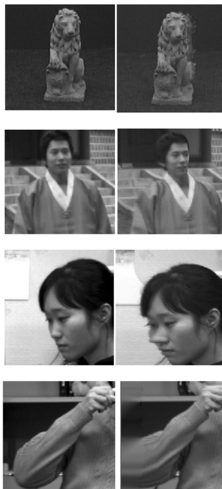
Fig. 1 Typical artifacts due to DIBR synthesis. Original images are in the left column and synthesized images are in the right column
