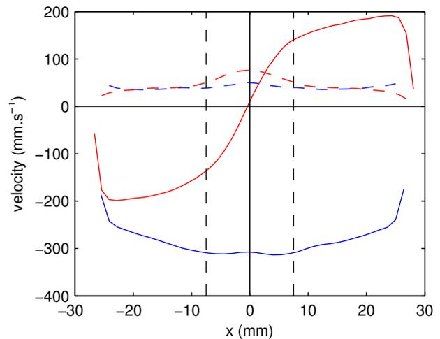
FIG. 4. Velocity profiles at  $z = -140\text{mm}$  along  $x$ -axis, for a flow rate of  $0.62\text{L}\cdot\text{s}^{-1}$  and a rotation rate of  $1.5\text{Hz}$ . Blue: vertical velocity  $u_z$  (solid line) and its standard deviation  $\sigma_{u_z}$  (dashed line). Red: tangential velocity  $u_y$  (solid line) and its standard deviation  $\sigma_{u_y}$  (dashed line). The vertical dashed lines stand for the core region of diameter 15mm.
