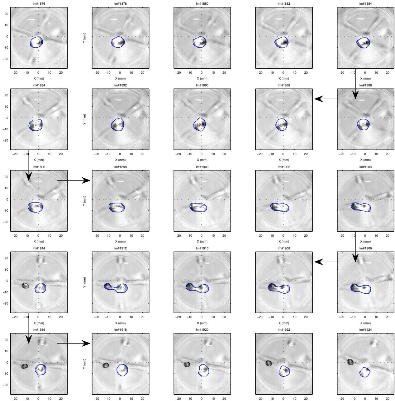
FIG. 15. Illustration of a breakup on case *B2*. Bottom view in the plane  $x - y$  (camera 2) with the detected contour in blue. One image over 2 is displayed and the time lag between each image thus corresponds to  $1/150\text{s}$  ( $(10f_2)^{-1}$ ). Please note that the sequence over reads from top left to top right then the second line reads from right to left, and so on, following the arrows.
