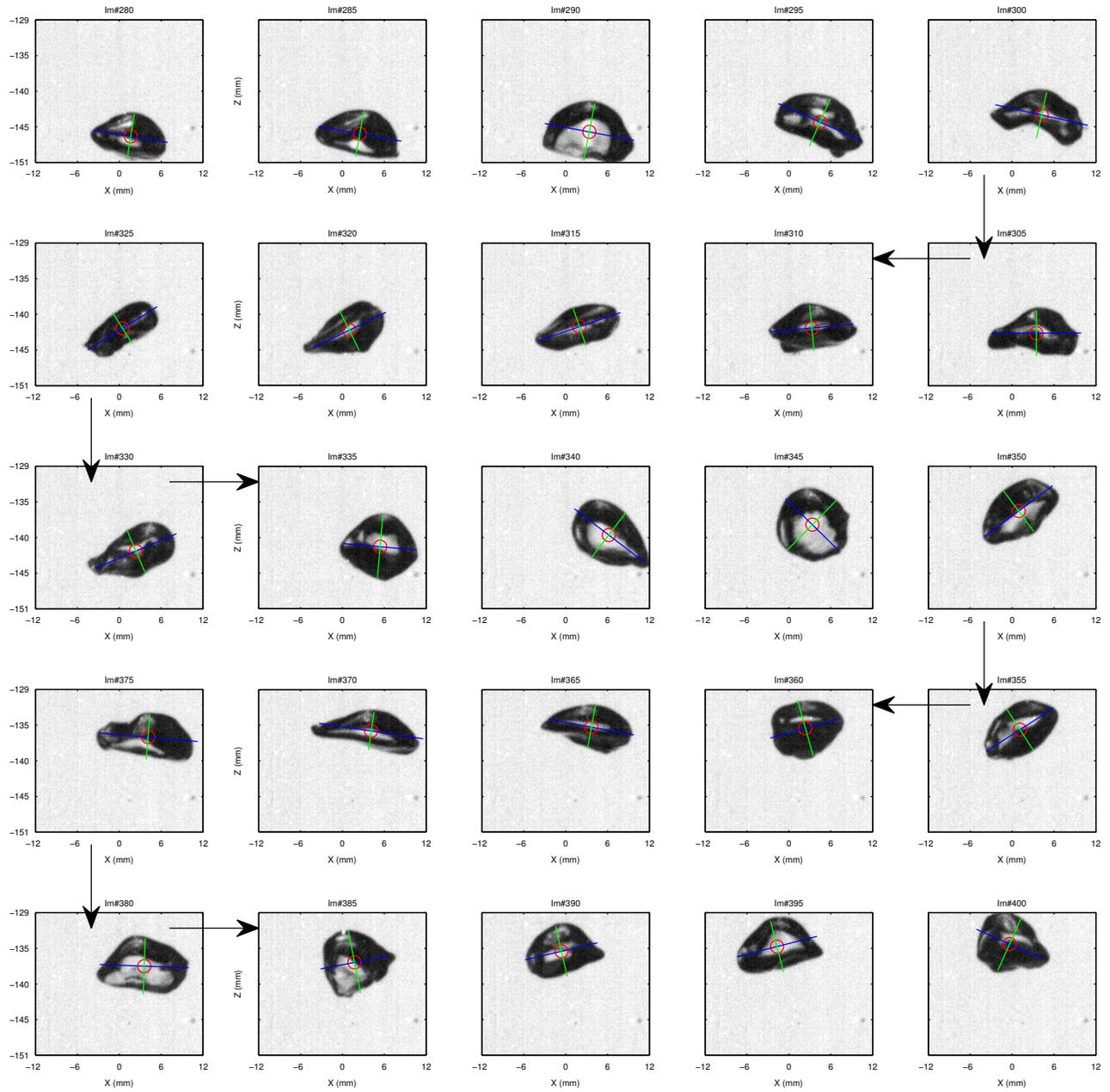
FIG. 8. Illustration of a deformation sequence on case  $B5$ . Side view in the plane  $x - z$  (camera 1) with the center of mass (red dot), the major (blue line) and minor axes (green line) of the equivalent ellipse. One image over 5 is displayed and the time lag between each image thus corresponds to  $1/60\text{s} \ ((4f_2)^{-1})$ . Please note that the sequence reads from top left to top right then the second line reads from right to left, and so on, following the arrows.
