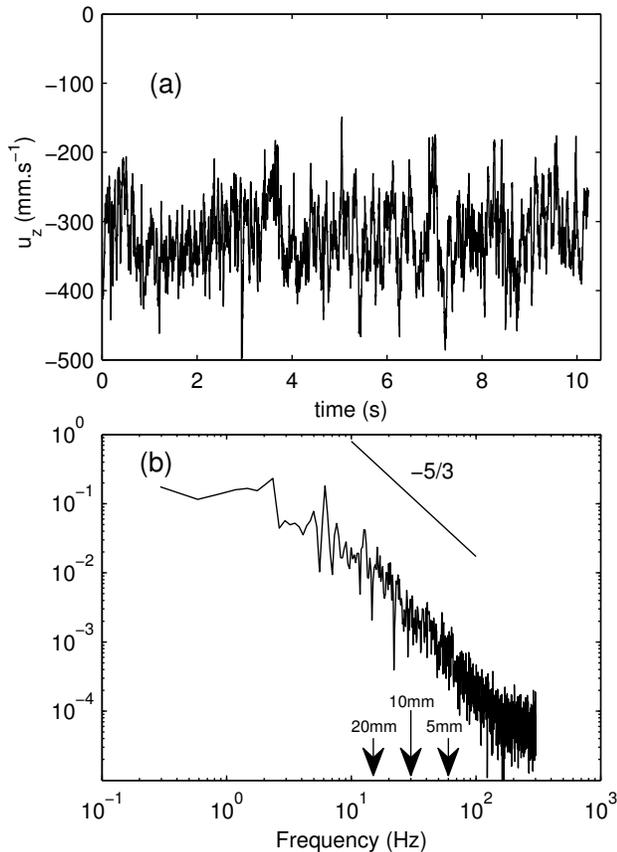
FIG. 6. Velocity measurements for a flow rate of  $0.62\text{L}\cdot\text{s}^{-1}$  and a rotation rate of  $1.5\text{Hz}$ . (a): time signal of the vertical velocity  $u_z$  at point  $x = -0.3, y = 0, z = -140$  (in mm). (b): corresponding power spectrum. Arrows stand for corresponding length scales using Taylor's hypothesis.
