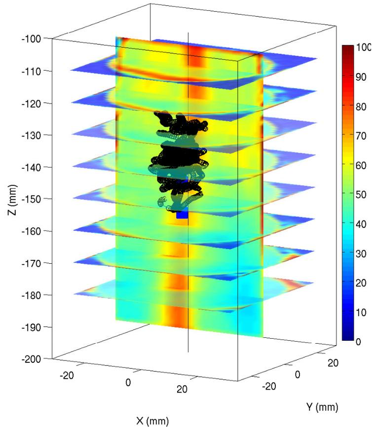
FIG. 5. Standard deviation of the velocity measured in one vertical plane and eight horizontal planes superimposed with the trajectory of bubble  $B5$  (black) and mean positions of the six bubbles (blue squares).
