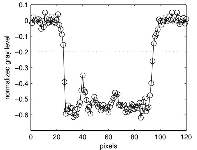
FIG. 2. Normalized gray level profile along constant height  $z = -146.5\text{mm}$  for view 1 of image 39 of sequence  $B5$  (see also top left quadrant in Fig. 3). Horizontal dotted line: threshold used for binarization. Bubble corresponds to values below the threshold. Calibration factor: 6.5 pixels corresponds to 1mm.
