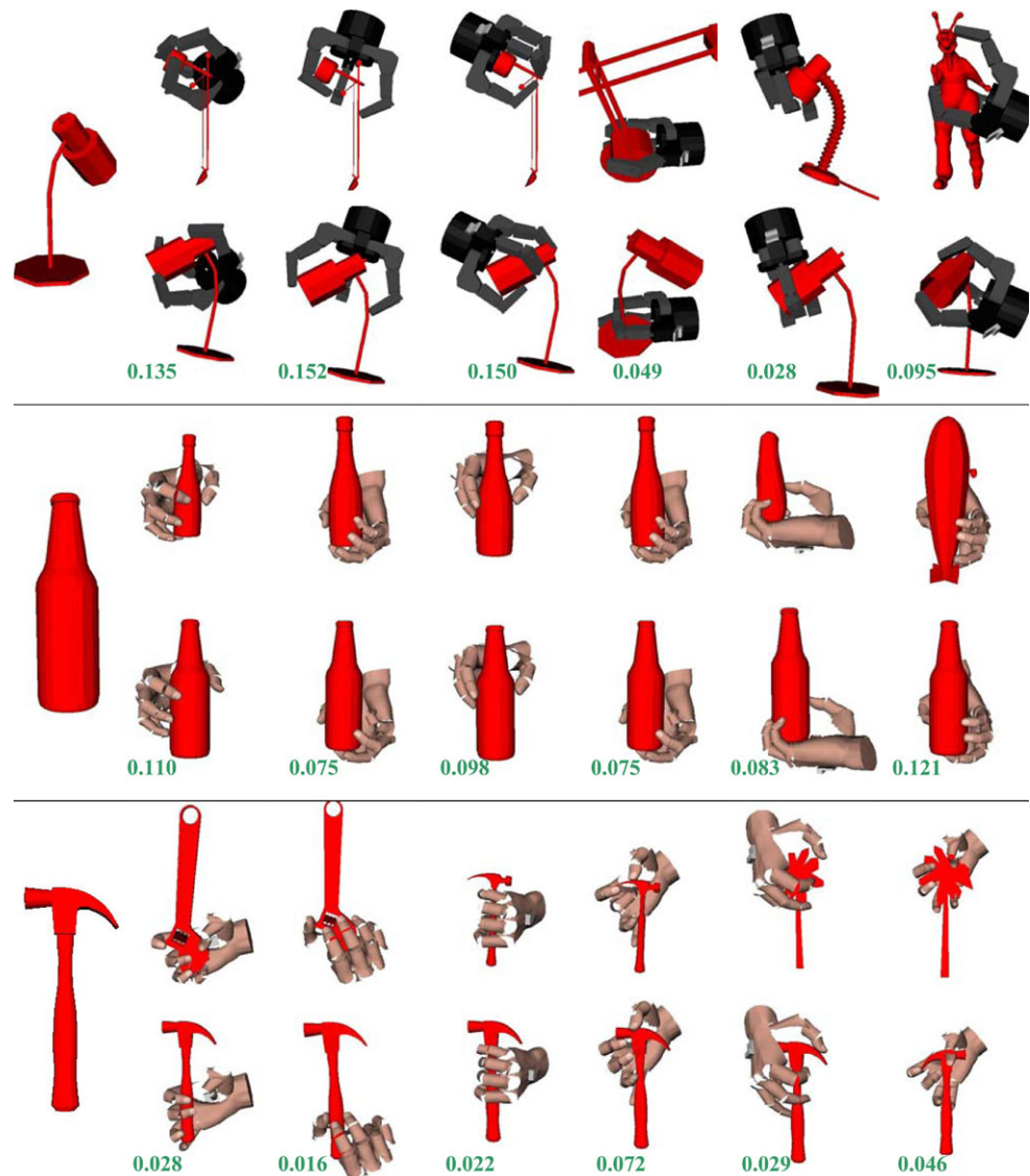
Fig. 1 Three example models and their grasps, using the database-backed planner with Zernike neighbors. For each model \alpha (left), the top row of images shows a neighbor from the database and a pre-computed grasp on that neighbor. Directly below each neighbor is the same grasp executed on \alpha , along with its grasp wrench space \epsilon quality measure (Ferrari and Canny 2002)
