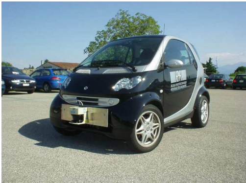
Figure 1. Modified Smart Car used at ASL. Observe the LMS 291 SICK laser sensor assembled on its front bumper.
