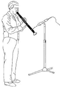
Figure 5. Clarinet recording. The microphone diaphragm axis is further off the instrument axis (on the picture to the right [4]).
