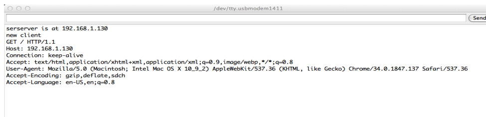
Fig 3.11c: Accessing shield as a client Figure 3.11a to 3.11c confirms working of shield as a server and PC as a client, after uploading the sketch in Arduino.
