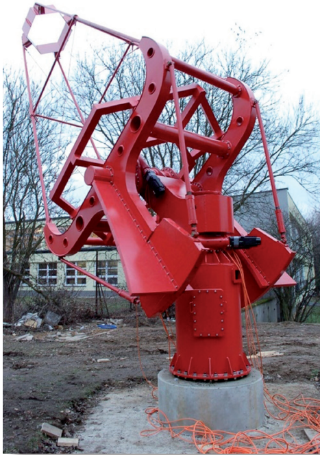
Fig. 2 The 4 m diameter D-C SST structure installed at IFJ PAN.
