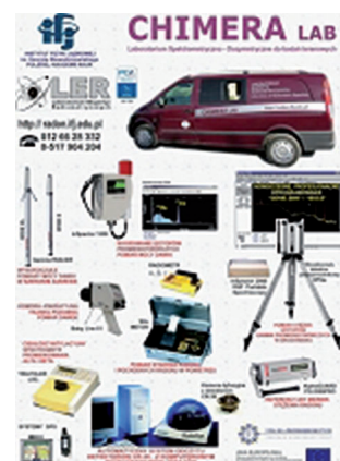
Fig. 2 The mobile CHIMERA radiometry laboratory and its basic equipment for measuring radon concentration, dose rates in the environment and for performing in situ spectrometry.
