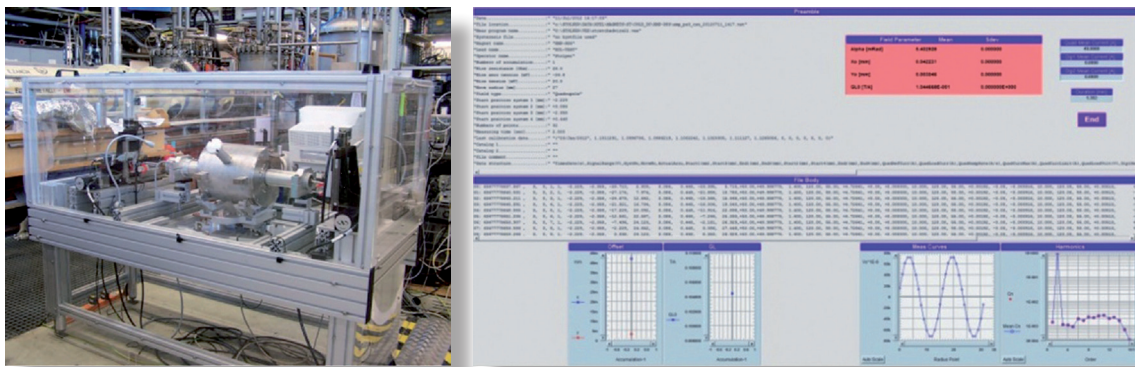
Fig. 11 Test of a warm quadrupole magnet and a screenshot of measurements performed.
