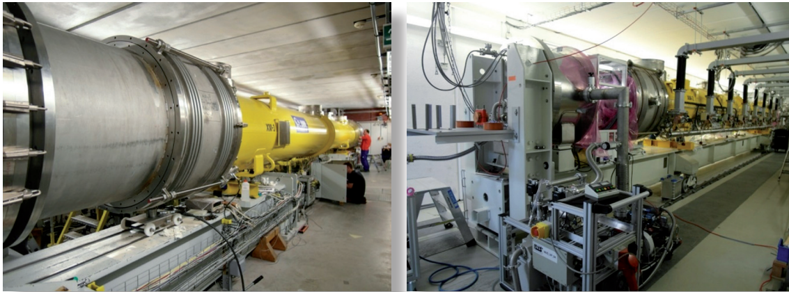
Fig. 16 Preparation of cryomodules for cold tests on the temporary test-stand (left) and on the final test-stand (right).
