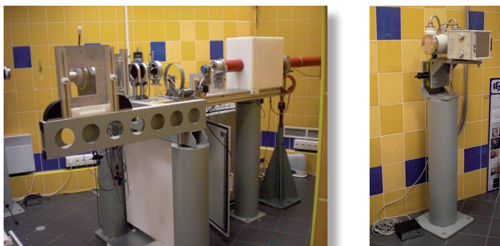
Fig. 4 Setup for proton ocular radiotherapy: beam forming bench and x-ray tube on an adjustable support.
