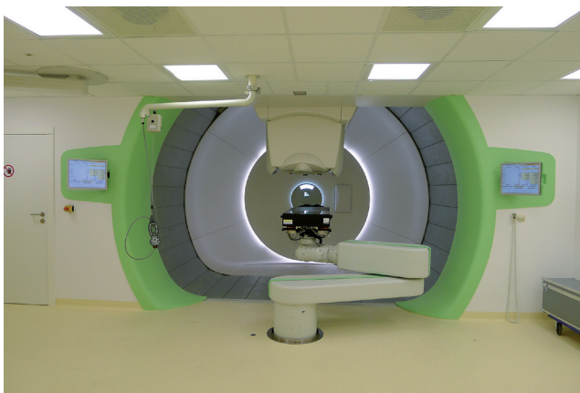
Fig. 7 View of the patient irradiation facility showing the gantry and the scanning beam nozzle (April 2014).
