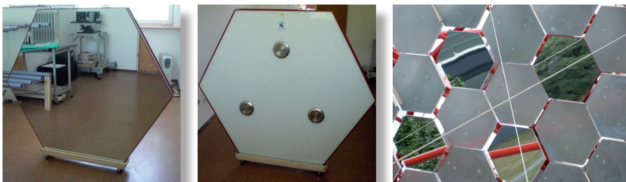
Fig. 3 Front and back sides of the MST mirrors (left and central); DAI mirrors mounted on the MST prototype (right).
