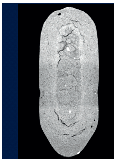
Fig. 13 \mu CT images after 2h hydration of originator and generic dosage forms.
