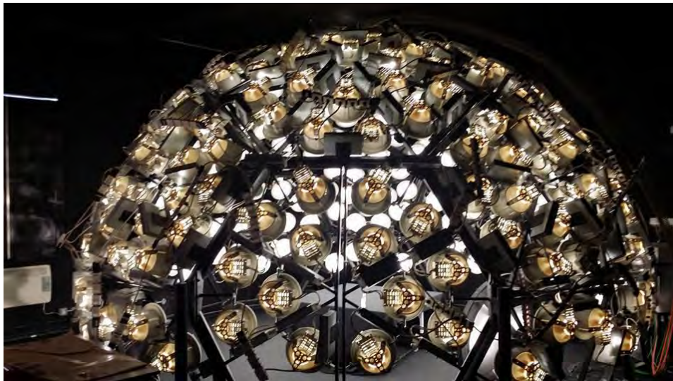
Figure 7.8 The Bartlett daylight simulator for scale models of buildings
