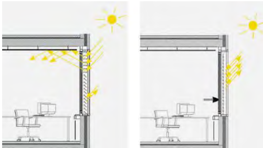
Figure 2.21 Shown an example application where louver can act as both daylight Light-redirecting ad shading system based on different inclination angles (Boubekri 2014).
