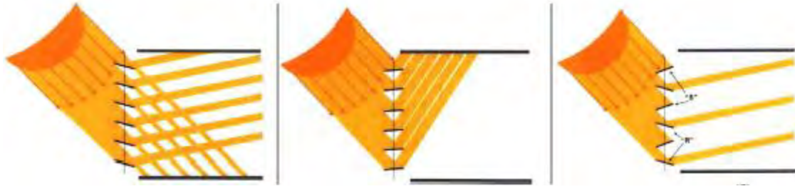
Figure 2.23 Louvers optimised for sunlight redirection, shading and combined system (McGuire 2005).
