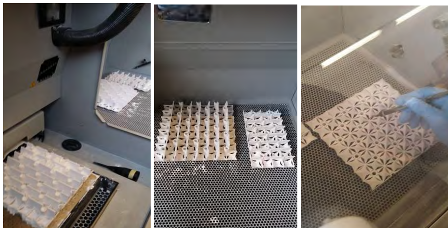
Figure 7.5 Final stage of depowdering the printed screens
