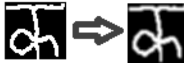
Figure 8. Applying the Filter to the Left Binary Image and Converting it to a Grayscale Image
