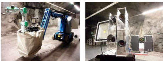
Figure 2. Images of the first functional prototype robotic vehicle for tunnel inspection. Left image: an overall image of the autonomous vehicle, the robotic arm and the imaging system; right image: the robot's sub-system of sensors, the cameras and the laser scanner.
