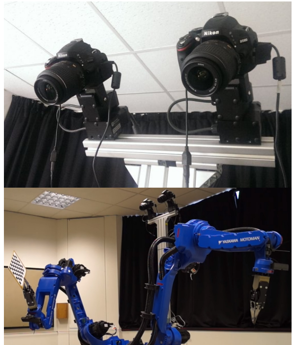
Fig. 1: Top: Our active binocular robot head. Bottom: Dual-arm Yaskawa robot with our robot head integrated.
