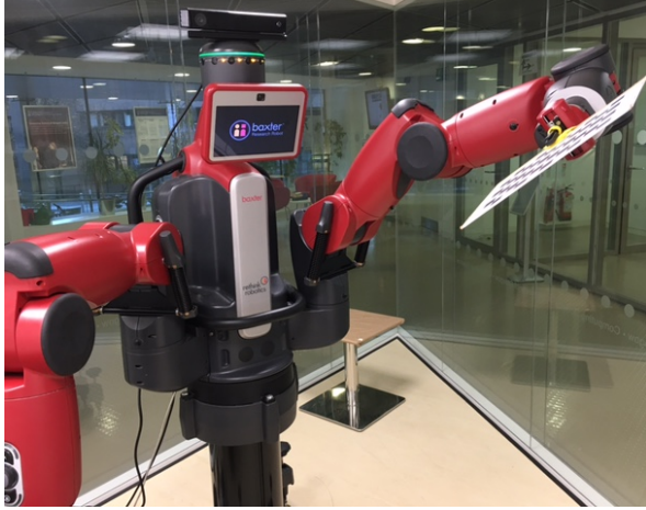
Fig. 2: Rethink Baxter robotic holdin the calibration target. In our experiments, we placed the RGBD camera (Kinect V2 in the figure) at the top of the robot’s head.
