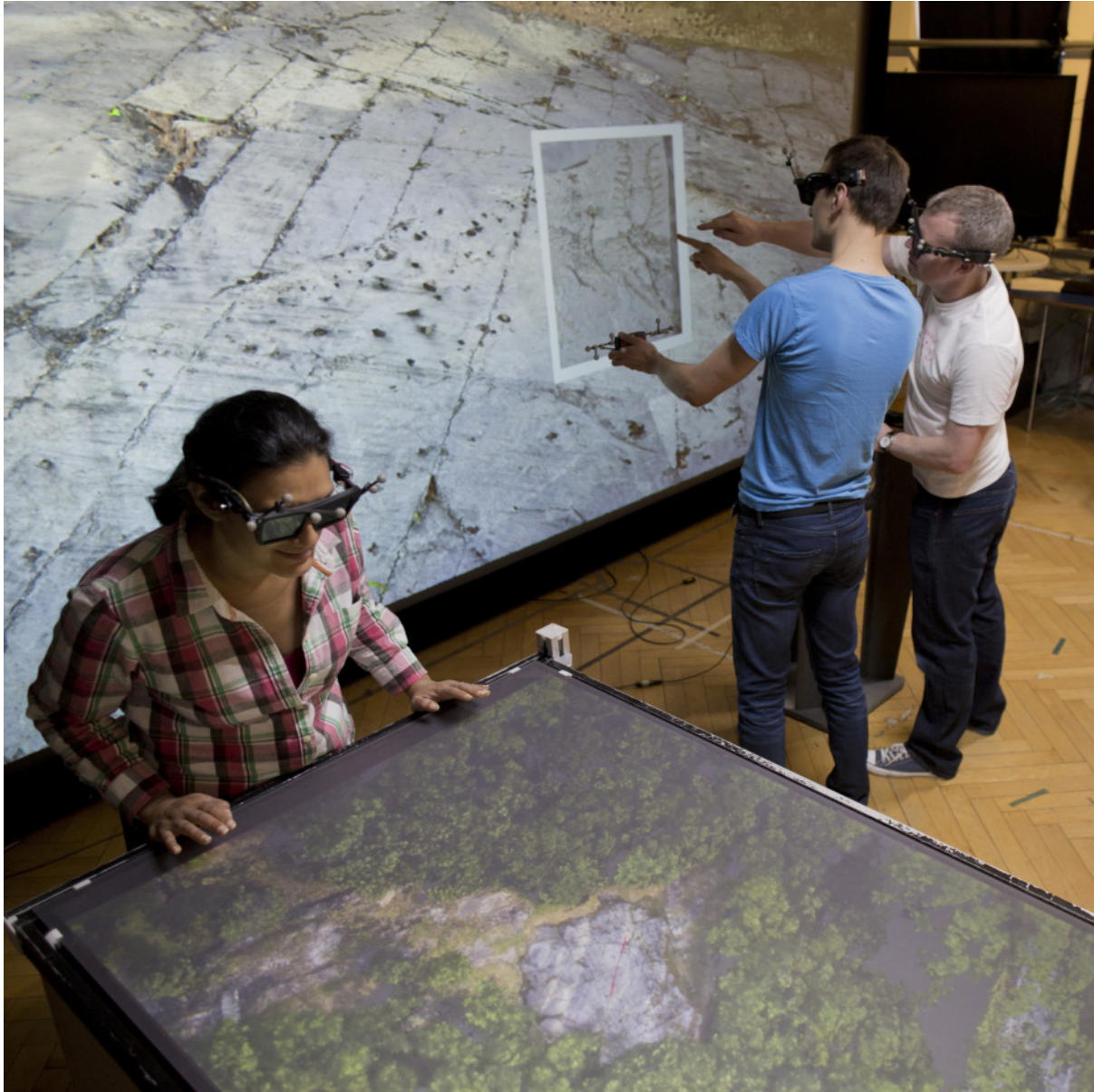
Figure 1. The 3D-Pitoti Scientists' Lab involves a large vertical multi-user 3D display (powerwall) and a multi-touch enabled multi-user 3D tabletop display. We use both displays for different subtasks of the data exploration. Handheld virtual 3D displays, called Photoportals, provide additional access points for individual or collaborative interaction with the data.
