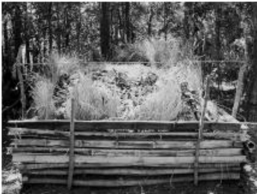
FIGURE 6 Aeta traditional built-up earthen charcoal pit kiln prior to ignition (photo by Nathaniel Salang).
