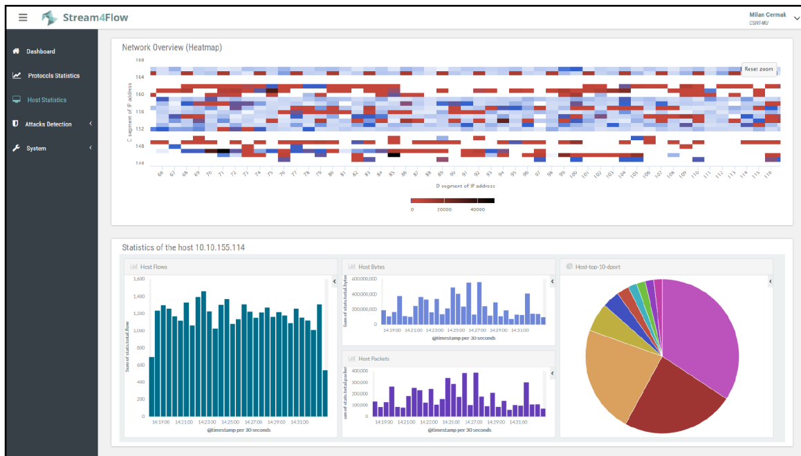
Figure 3. Stream4Flow web interface with network overview and detailed characteristics of a selected host.
