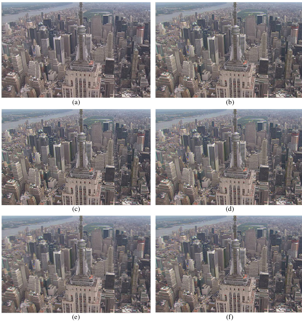
Fig. 9 Comparison of subjective quality of decoded frames ( city sequence, 118th frame, QP22) (a) \text{TCR}_{\text{Level}} = 0 (maximum complexity), (b) \text{TCR}_{\text{Level}} = 2 , (c) \text{TCR}_{\text{Level}} = 4 , (d) \text{TCR}_{\text{Level}} = 6 , (e) \text{TCR}_{\text{Level}} = 11 , (f) \text{TCR}_{\text{Level}} = 14 (minimum complexity).
