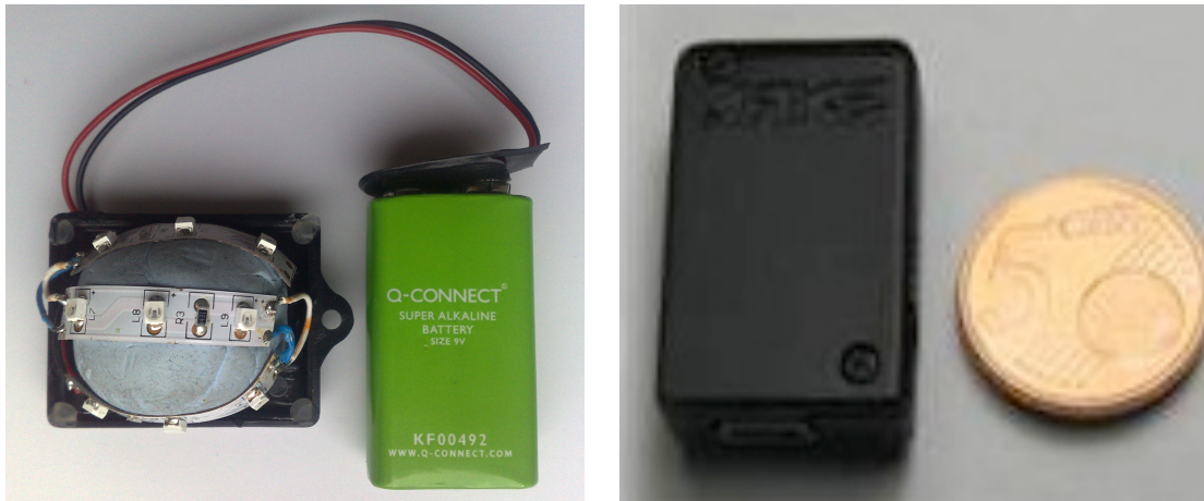
Fig. 1. (a) IR tag with 9V battery attached, (b) JAKE sensor pack shown with a five cent euro piece.
