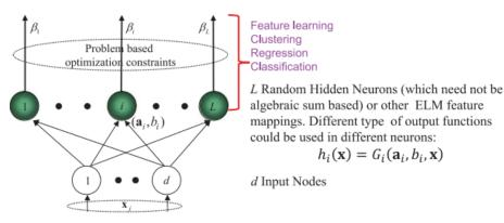
Figure-1. ELM Architecture (Huang et al., 2015).
