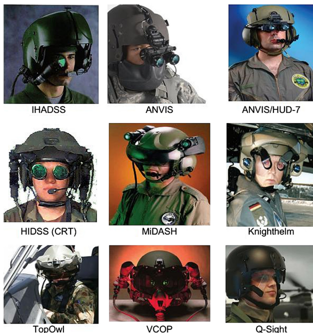
Fig. 19 Selected current and future rotary-wing HMD programs.
