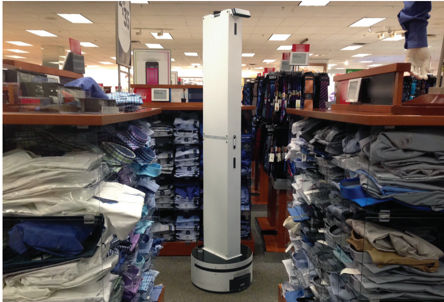
Fig. 2. AdvanRobot in operation in a store. At the bottom, the lower circular part is the robotic base. On top of it, the RFID system, which is foldable. Finally, at the top of the RFID system the RGBD camera for obstacle detection.
