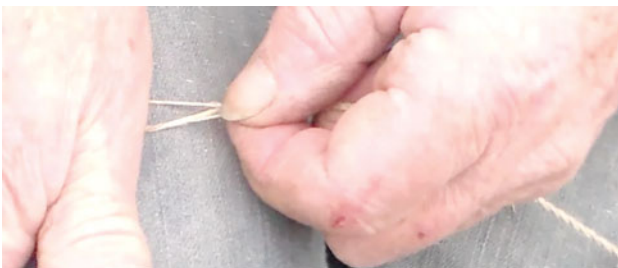
Figure 7. CTM(1): Twisting dried flax into twine.
