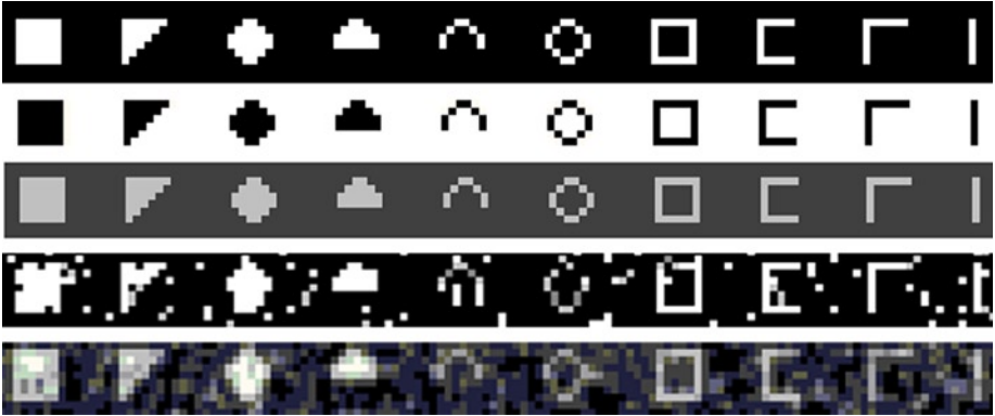
Figure 7-8. Portion of the synthetic interest point alphabet: points, edges, edges, and contours. (Top to bottom) White on black, black on white, light gray on dark gray, added salt and pepper noise, added Gaussian noise
