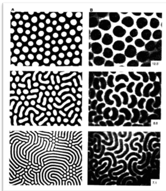
Figure 2: Frustrated phase separation in different systems magnetic and organic thin films (From ref.5)
