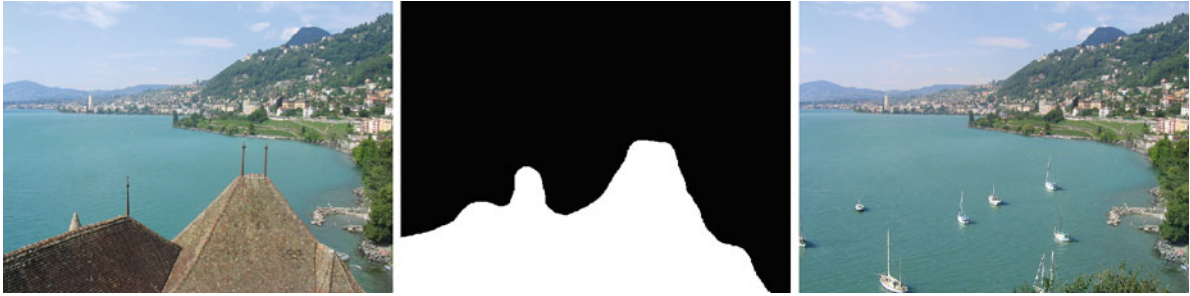
Inpainting, Fig. 17 Left: original image. Middle: inpainting mask \Omega , in white. Right: inpainting result obtained with the method by Hays and Efros [18], images taken from their paper
