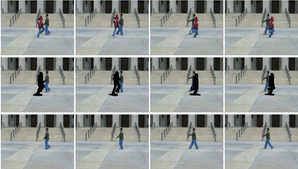
Inpainting, Fig. 16 Top row: some frames from a video. Middle row: inpainting mask \Omega in black. Bottom row: video inpainting results obtained with the algorithm of Patwardhan et al. [25]
