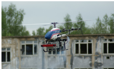
Fig. 1: Unmanned helicopter ARTIS of DLR (German Aerospace Center).
