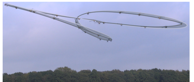
Fig. 5: Ground camera perspective of the flight test of the clover leaf path flown without position feedback.
