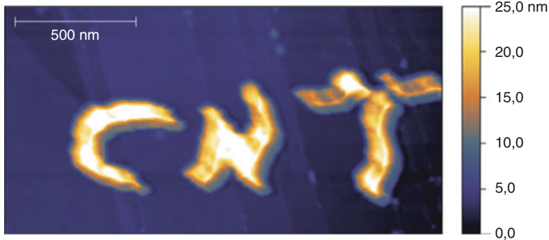
Robot-Based Automation on the Nanoscale, Fig. 7 Multiwalled carbon nanotubes on HOPG substrate manipulated by the AFM. When moving the AFM tip laterally, the height control loop was turned off in order to avoid slipping of the AFM tip over the CNT. It could be
