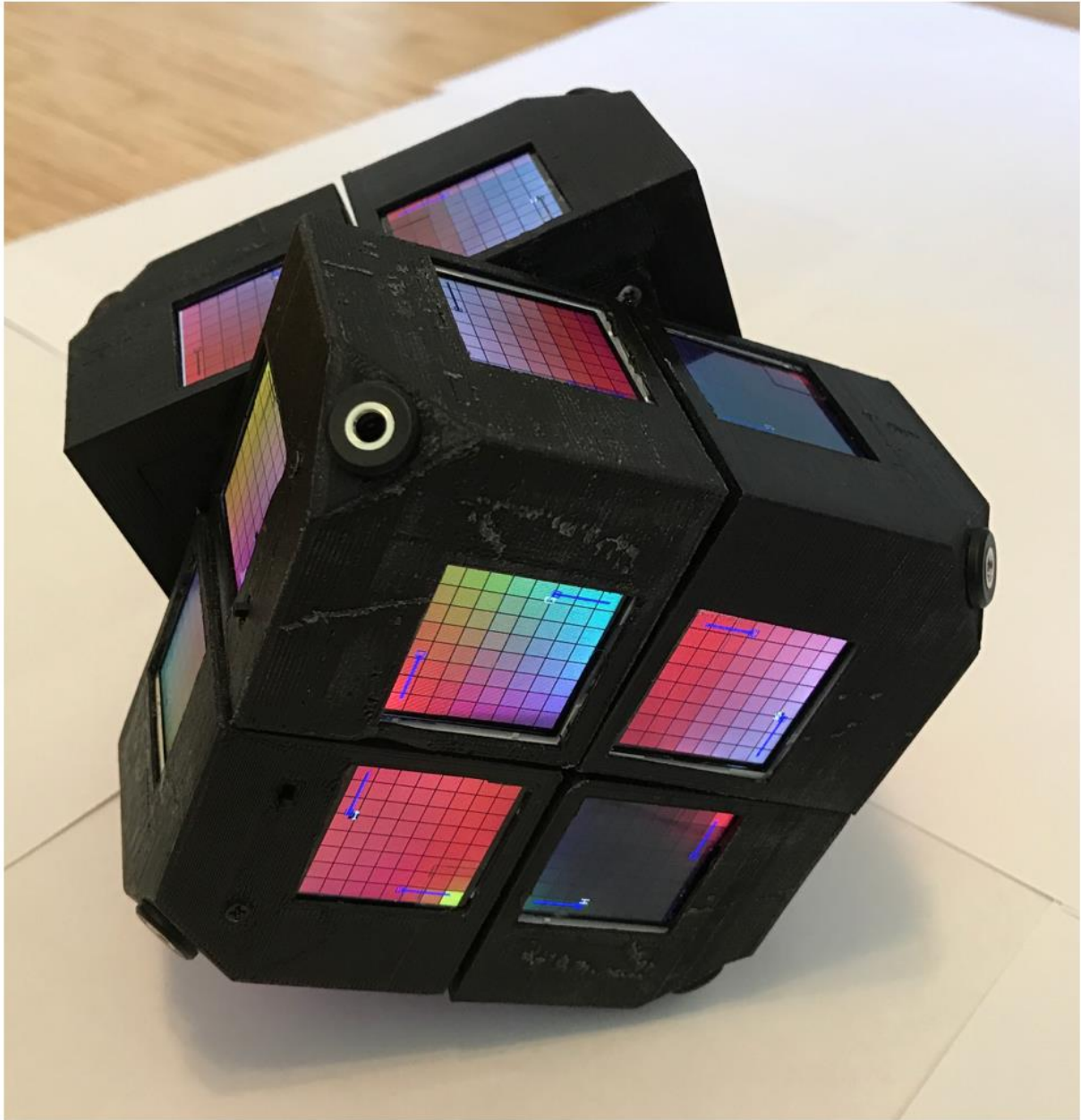
Figure 6. The assembled and functional prototype Cubios of 8-elements
