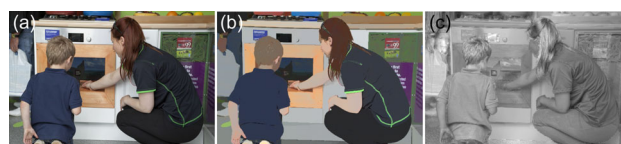
Figure 1 (Color online) Example of image decomposition. (a) Input image; (b) reflectance; (c) shading.
