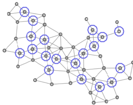
Figure 6. Graph of 50 vertices. Vertices in the T_2 -CDS are marked in blue.
