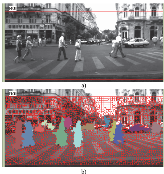
Figure 2: Obstacles detection: a) intensity image ROI; b) corresponding superpixels-based detected obstacles (with random color for each obstacle).
