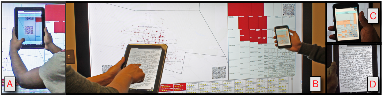
Figure 1. The Visfer framework enables transferring visualizations across devices to support cross-device visual sensemaking. (A) User captures a QR code; (B, C, D) visualizations loaded on personal devices from the large display. Transferred visualizations are adapted to the target device.
